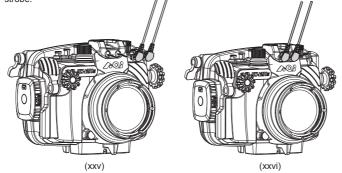
c. The flash trigger signals (electrical signals) will be transferred from the camera Hot Shoe to the Multi-control Device through the Hot Shoe Connector (included in the package). The Optical Flash Trigger in the Multi-control Device will convert the electrical flash triggering signals into optical signals and then will deliver them to the Fiber Optic Cable. The Fiber Optic Cable (not included in package) picks up the optical signals and delivers them to the external strobe.
