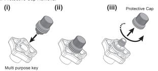
b. Mount the Vacuum Valve to the M16 Port on the housing
